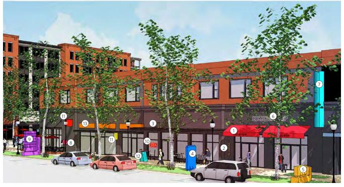
Figure 19.2 Diagram of Standard Signage Placement
